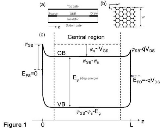
**Fig.1:** Geometry and band diagram of the GNR-FET: (a) cross-section, (b) top view of the armchair shaped edge GNR forming the channel, and (c) sketch of the spatial band diagram along the transport direction.
