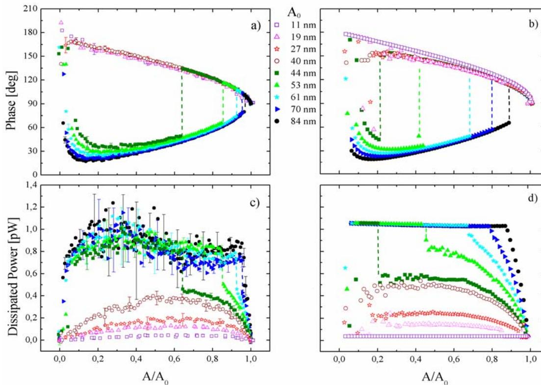
**Figure 1a-d:** Experimental (1a) and calculated (1b) phase shift and experimental (1c) and theoretical (1d) dissipated power versus the oscillation amplitude obtained as the tip-sample distance is reduced. Symbols correspond to different free oscillation amplitudes  $A_0$ . Experimental data were smoothed (average over 10 data points), the standard deviation is shown.
