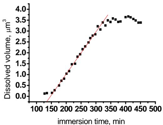
Fig. 3. Kinetics of dissolution of aluminum matrix near Fe-rich intermetallic on AA5083 during immersion in 0.05 M NaCl solution.
