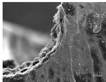
Figure 4. Edge of a microreactor channel coated with CNF layer
