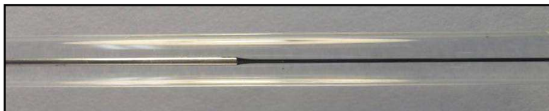
Fig. 1 : Injection of a nanotube dispersion in the co-flowing stream of a PVA.
