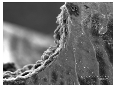
Figure 4. Edge of a microreactor channel coated with CNF layer
