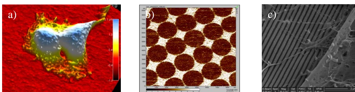
Figure 1: a) Topography image taken by an AFM of mesenchymal stem cells adhered on a glass surface; b) Phase contrast AFM image of a micro-contact printed self assembled monolayer obtained with a force modulation mode of operation; c) SEM image of cells on a microstructured polymer (Courtesy of Dr. Elena Martínez, IBEC).
