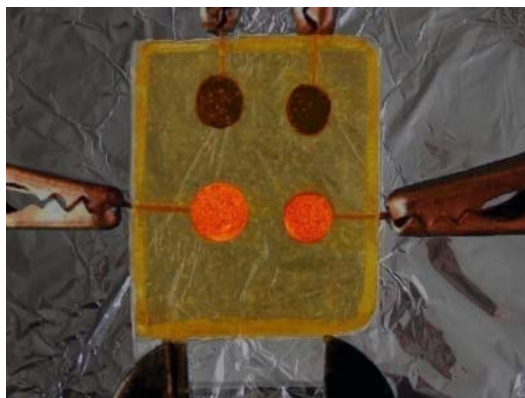
Red-emitting device, suitable for large area manufacturing, promising for use in illumination of plants in greenhouses.
