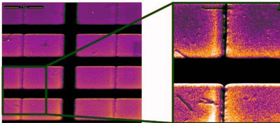
TMV particles inside a polymer resist grid (PMMA). The particle at the bottom can be separately addressed by two liquid containers (left and right). Grid size: 4.1x2 μm
