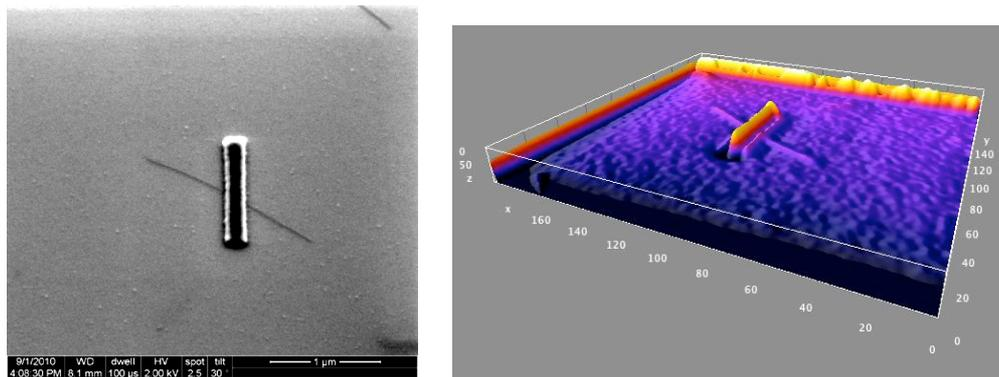
TMV particle covered by a rectangular block of polymer resist (mrEBL6000.1). Image size: 3.7x3.4 μm
