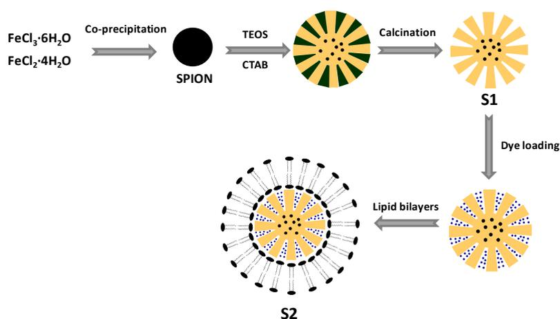
**Figure 1.** Synthesis of superparamagnetic core-shell nanoparticles.
