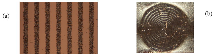
Figure 1.(a) Al nano-particle pattern with period \Lambda=17 \mu\text{m} obtained after sinusoidal illumination with a high contrast light pattern. The particles are deposited from an hexane suspension (b) \text{CaCO}_3 micro-particle ( d=1-3 \mu\text{m} ) pattern deposited in air under a 2D light pattern of concentric circular fringes
