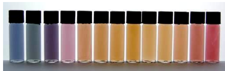
Figure 1: Synthesised AuNR solutions with longitudinal modes between 625nm (left) and 925nm (right). The longitudinal mode increases by 25nm between bottles.
