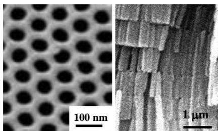
**Figure 1:** Top view (left) and transversal view (right) of a NAA structure formed by the periodic repetition of two layers with different refractive index and thickness (SEM image).
