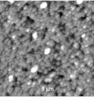
SEM image of etched steel and AFM image of surface for micrometre (0,51 $\mu$ m Ra) and nanometre roughness observation (16 nm Ra).
