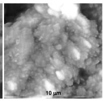
SEM image of etched aluminium and AFM image of surface for micrometre (2,5µm Ra) and nanometre roughness observation (136nm Ra).
