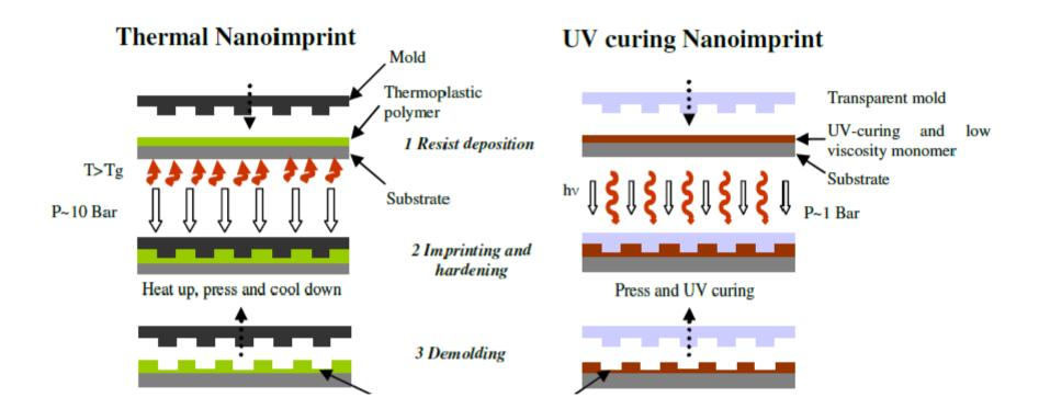
Si Master stamp was replicated on OMS (UVNIL). Afterwards the mould was used for texture replication on polymeric material (Thermal NIL).
