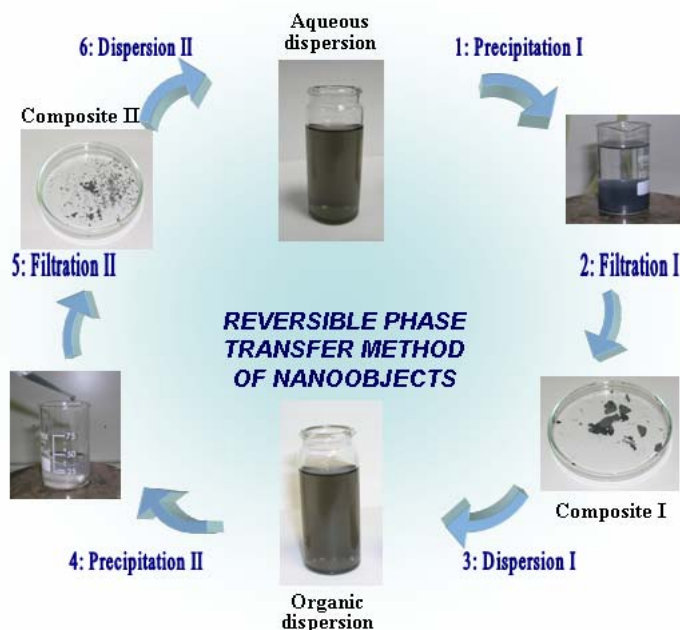
Figure 2. Method for the reversible transfer method of nano-objects between aqueous and organic phases using polymeric ionic liquids
