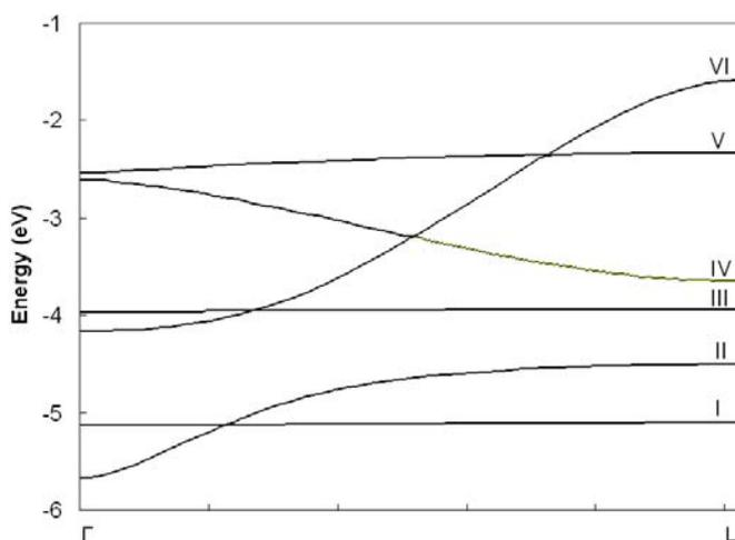
**Fig. 2** The electronic band structure of the linear polymer  $(\text{AuAl}_4\text{Au})_{\infty}$ . The Fermi level is at -3.95 eV.
