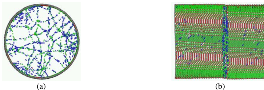
Fig. 6. a) Cross section of the D_c=20 nm nanowire for \gamma=0.04 showing the GND dislocations that form a disordered twist sub-boundary. See Figure 5 for the colour code. b) Side view.
