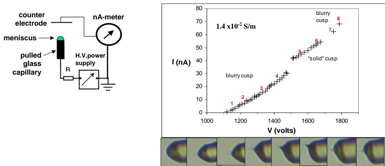
Figs 3 (left) and 4: Transmitted current vs. voltage for two different electrical conductivity solutions. (Fig.3:  $i_d=5.5$   $o_d=14$ . Fig.4:  $i_d=4.5$   $o_d=10$ , in  $\mu\text{m}$ . Counter electrode= porous plate.)
