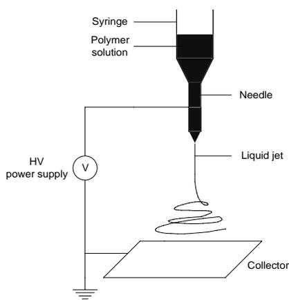
Figure 1 – Schematic illustration of a typical electrospinning setup.
