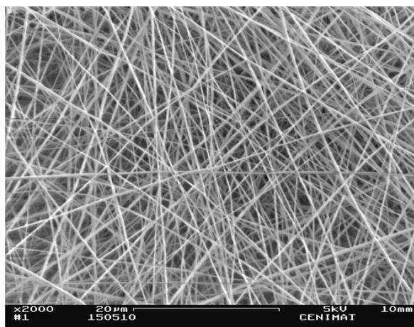
Figure 2 – Typical SEM image of the nonwoven mat of cellulose acetate nanofibers.
