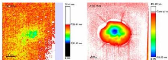
Figure 3. Results obtained after indenting a bump. Mechanism shown at different load with modulus mapping of the surface after the indent.
