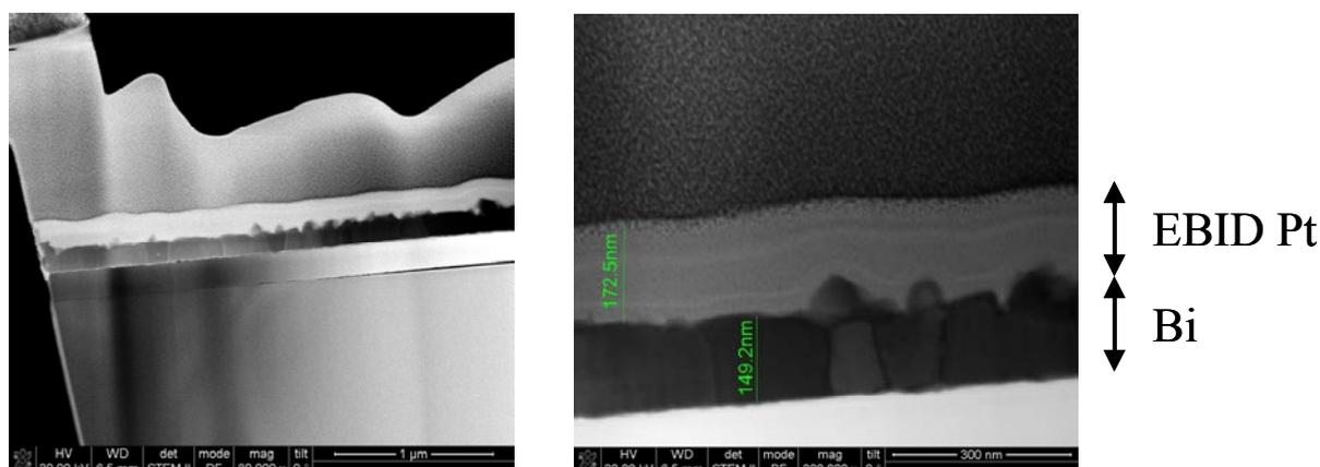
**Figure 2.** In-situ STEM images under 30 keV of a lamella prepared inside our dual-beam equipment from a Bi thin film grown by thermal evaporation on a  $\text{Si}_3\text{N}_4//\text{Si}$  substrate. The left picture is a dark-field STEM whereas the right one is a bright-field image.
