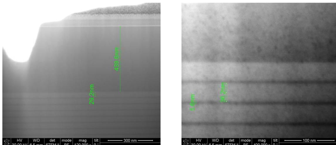
**Figure 1.** In-situ bright-field STEM images under 30 keV of a lamella prepared inside our dual beam equipment from a GaAs/GaAsAl multilayer grown by MOCVD.
