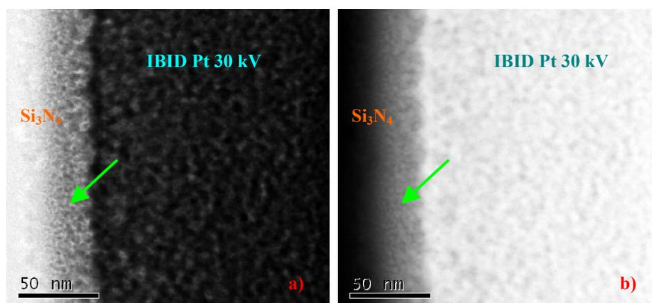
**Figure 3.** In-situ STEM images under 30 keV of an ion-beam-induced deposit of Pt grown on a  $\text{Si}_3\text{N}_4//\text{Si}$  substrate in our dual-beam equipment. The left picture is a bright-field image whereas the right one is a high-angle-annular-dark-field image.
