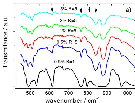
Figure 1. FTIR spectra of PVDF-CNF nanocomposites with different CNF concentrations.
