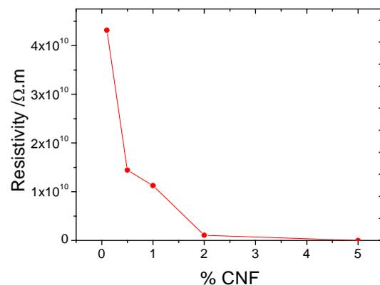
Figure 2. Electrical bulk resistivity of the CNF-PVDF nanocomposites as a function of CNF volume concentration.
