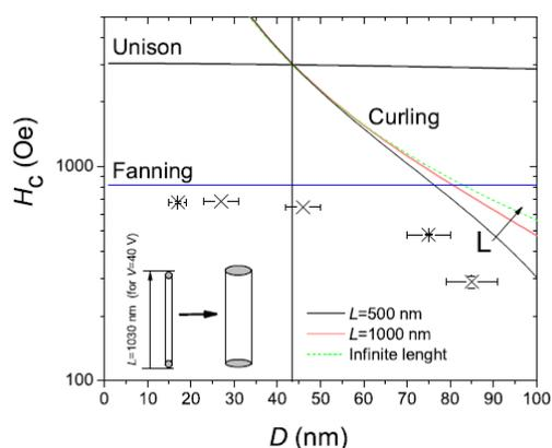
Fig. 3. Coercivity evolution for samples with different diameter. Nucleation field predictions for the diverse reversal modes in samples with a finite length of 1000 nm (length that correspond with sample prepared at 40 V and filled during 10 min) are shown. The vertical line signals the critical diameter  $D_{cr}$ . The different curves for curling correspond to wires with various lengths.
