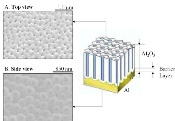
Fig. 1. Schematic drawing of the nanoporous alumina structure as obtained as a result of anodic oxidation. Example of the top view (A) and the side view after aluminium removal (B) of a sample synthesized at 160 V during 2 hours in  $\text{H}_3\text{PO}_4$  1%.
