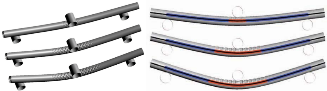
Figure 1: Twisted MWCNTs. (a) Strain energy vs twisting angle log-log plots for various MWCNTs and (b) data collapse upon appropriate rescaling. The power-law fits with exponents 2 (blue) and 1.63 (red) are shown for illustration. (c) Rescaled torque vs twisting angle relation highlighting the unified law. (d) 35-walled CNT in torsion, deformed shape (top), Gaussian curvature map (middle, green is zero, red is positive, blue is negative), and energy density map (bottom, red is high, blue is low).
