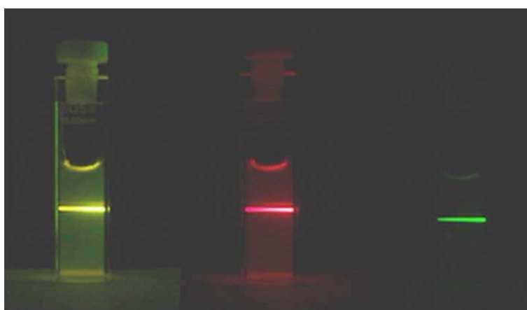
Dispersion of rhombic \text{Er,Yb:YF}_3 nanophosphors (sample R) in water showing UC luminescence sample when excited at 980\text{ nm} : (left) total UC, (center) UC viewed through a red filter, (right) UC viewed through a green filter. The photograph has been taken using a LUMIX DMC-digital camera (1 second exposure at ISO 400).
