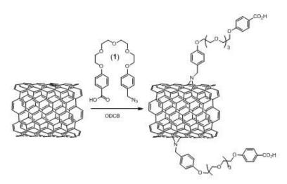
Functionalized SWNT were characterized by analytical, spectroscopic such Raman, UV/Vis, XPS and NMR techniques. The Raman spectra taken both in aqueous dispersion and in the solid phase indicated modification of the SWNT backbone. These simple functionalized SWNTs are promising for attaching other functional groups, amino acids, and DNA to nanotube for chemical and biological applications.
