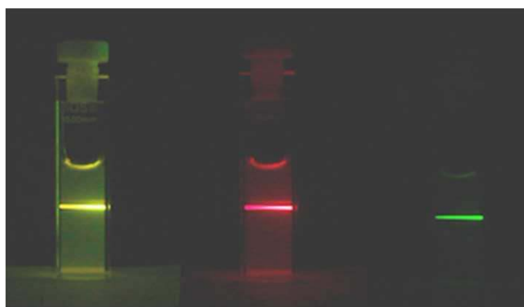
Dispersion of rhombic \text{Er,Yb:YF}_3 nanophosphors (sample R) in water showing UC luminescence sample when excited at 980 nm: (left) total UC, (center) UC viewed through a red filter, (right) UC viewed through a green filter. The photograph has been taken using a LUMIX DMC-digital camera (1 second exposure at ISO 400).
