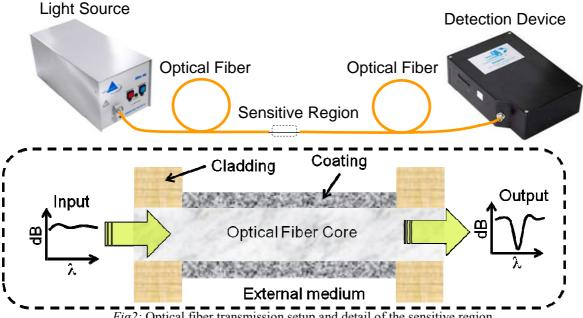
Fig2: Optical fiber transmission setup and detail of the sensitive region.
