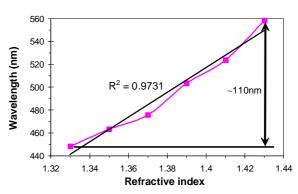
Fig4: Resonance wavelength shift as a function of the external refractive index.
