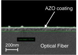
Fig1: SEM image of an AZO coated optical fiber.
