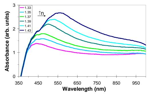
Fig. 3: Absorbance spectra obtained when the sensitive region was immersed in different glycerin/water concentration solutions of refractive indices 1.33, 1.35, 1.37, 1.39, 1.41, 1.43.
