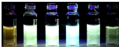
Fig. 3- Colour of the CdS QDs with different pH
