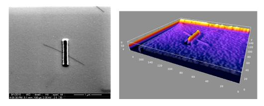
TMV particle covered by a rectangular block of polymer resist (mrEBL6000.1). Image size:  $3.7x3.4 \mu m$
