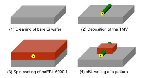
Virus nanotube immobilization through negative resist mrEBL6000.1 (fabrication)
