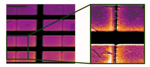
TMV particles inside a polymer resist grid (PMMA). The particle at the bottom can be separately addressed by two liquid containers (left and right). Grid size:  $4.1x2~\mu m$
