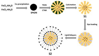
Figure 1. Synthesis of superparamagnetic core-shell nanoparticles.
