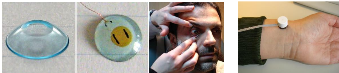
Figures. Examples of biomedical prototypes made with the piezoresistive thin film
