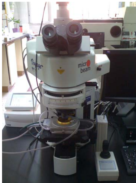
Figure 2. Confocal micro-Raman spectrometer and high temperature stage system (Linkam TS1500 with a T95 system controller) used for the experiments.
