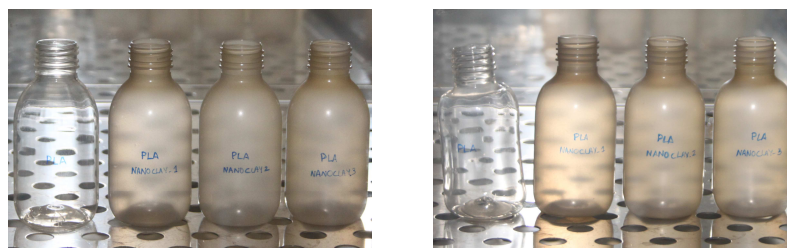
Figure 1. Picture of the PLA, PLA_3%Clay1, PLA_4%Clay1 and PLA_5%Clay1 bottles from left to right before (left side) and after (right side) a thermal treatment at 60 °C.
