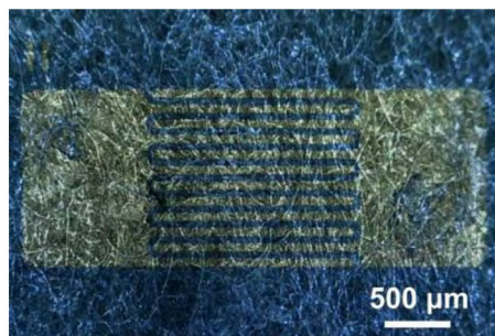
Figure 1: Optical micrograph of a WS 2 photodetector on paper. Figure 2: Photoresponse performance of the WS 2 device.
